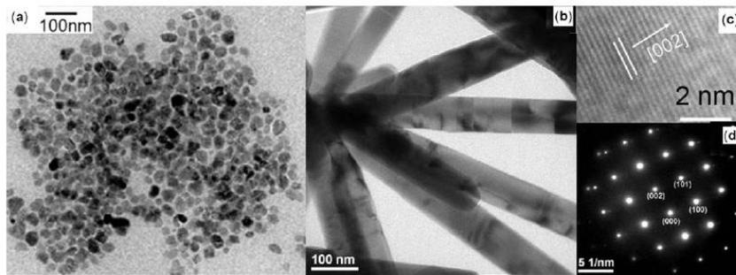
Growth of ZnO nanorods from solution using low temperature route (~80C) on nanoparticle seeded substrates. (a) TEM image of the seed nanoparticles taken on a grid from a suspension in ethanol,
