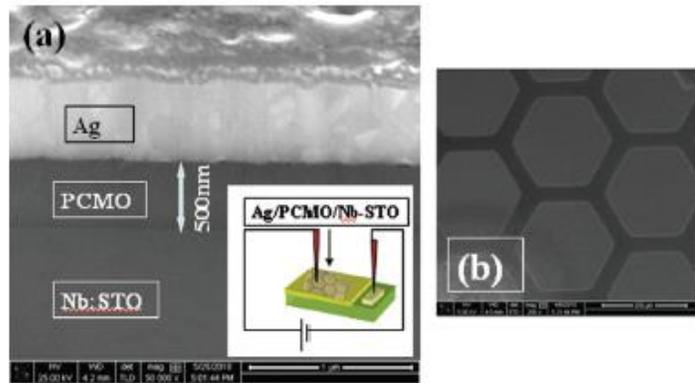
PLD grown multilayers of manganites (PCMO) on Nb:STO single crystalline substrate.
