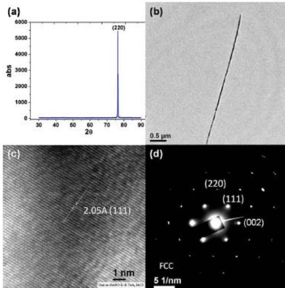
FCC metal nanowires grown by electrode position in AAO templates. (a) XRD pattern of 55 nm diameter nanowire arrays, (b) TEM image of a 55 nm diameter nanowire, (c) HRTEM image of the lattice planes in a 55 nm diameter nanowire, and (d) the electron diffraction pattern of a 55 nm diameter nanowire.
