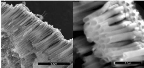
Cu nanotube grown by electro-deposition in rotating electric field.
